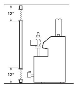
Fig. 3: Location of Openings for Combustion/Ventilation Air
